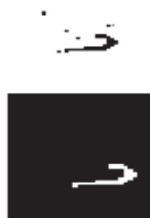
Figure 7. A sample handwritten character with noise (above) and after applying averaging and median filters (below)
