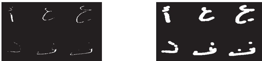
Figure 8. Dilation process effect on the character image; characters before dilation (above), characters after dilation (below)
