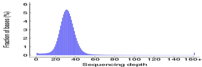
**Figure 5.** Sequencing depth histogram. The X-Axis is the sequencing depth, and Y-axis means the rate of the sequencing depth.
