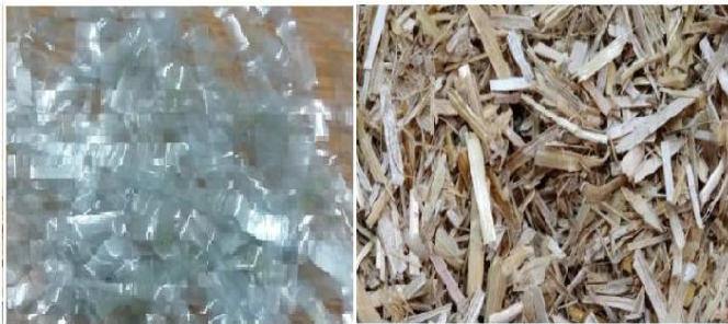
Figure 1: Plastic Fibers and Barley Straw Materials
