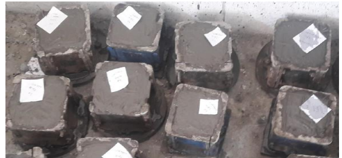
Figure 2: Casting of Cubes
