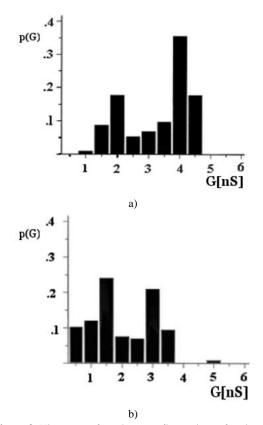
Figure 3. Histogram of conductance fluctuations of porin and EF-porin. The applied potential was +10 mV; T = 20 °C.
