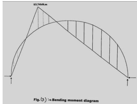
Two-hinged arch is the statically indeterminate structure to degree one. Usually, the horizontal reaction is treated as the redundant and is evaluated by the method of least work. Towards this end, the strain energy stored in the two-hinged arch during deformation is given. The reactions developed due to thermal loadings are discussed. Finally, a few numerical examples are solved to illustrate the procedure. ({11}, {13}, {12}).
